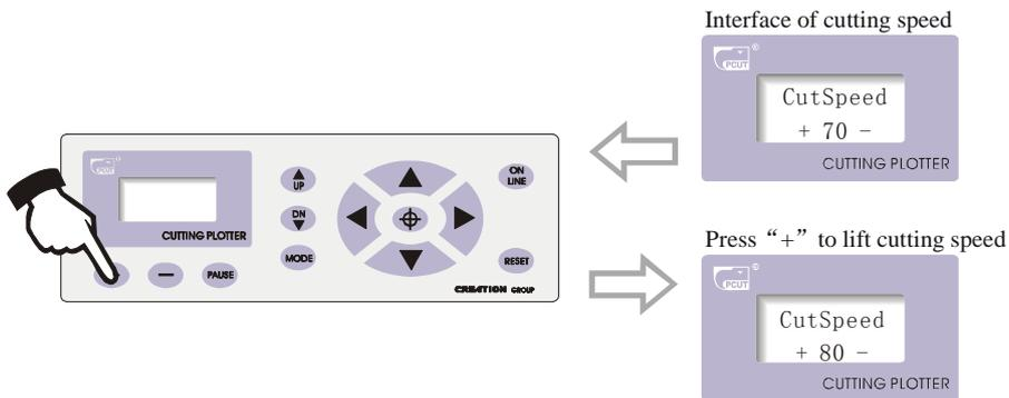
➤ When cutting at high speed, curve may look zigzag, but it is not a trouble, lowering the speed will eliminate the indention.
