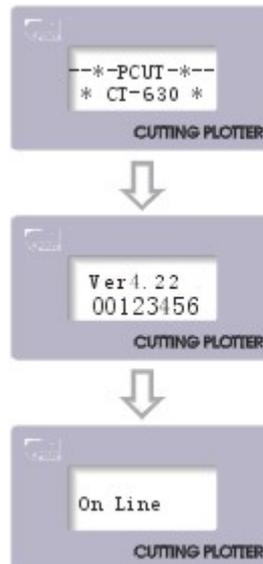
6.2.1.4 When the initializing is over, the machine is in online state and connectable with the computer to be operable.
