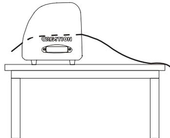
6.2.2.3 Adjust horizontal position of paperweight wheel according to width of paper. a distance of minimum 1-10CM is set between paperweight wheel and paper edge to ensure good running of paper.
