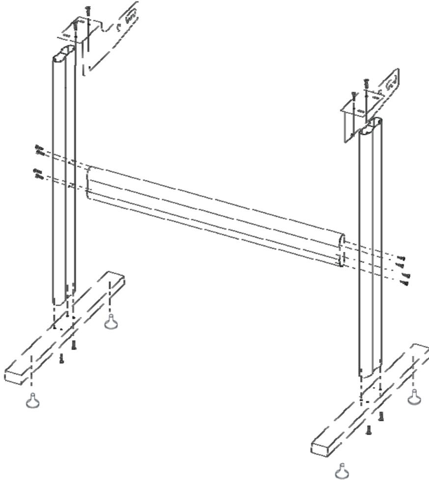
Take parts of the foot stool out of the pack, open the parts bag, install the foot stool as the map shows. After installation place the host on the support with screw hole targeted, then fasten it with screw.
