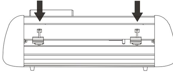
6.2.2.2 Insert the media into the space between paperweight wheel and main shaft, and pull out the media to appropriate length from the front of the host.
