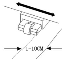
6.2.2.4 Raise two handles of paperweight wheel, to make paperweight wheel down to press paper.
