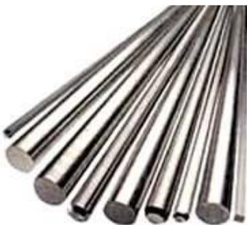
Each axis travels on a pair of  $3/8$ " precision steel rods. It is critical that these rods are smooth and without scratches or nicks as these marks will severely reduce the life of the bearings. Small imperfections may be removed carefully with emery cloth or very fine sandpaper (600 grit or finer). Rods with any blemish that cannot be removed by fine sanding or polishing should be discarded and replaced.
