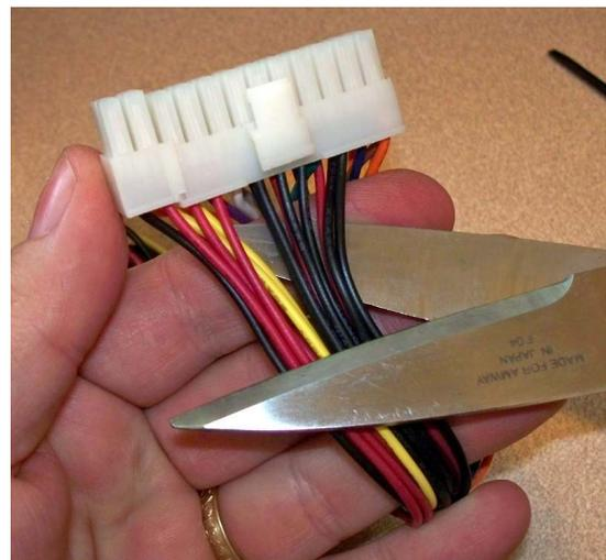
With all of the black, red and yellow wires separated from the harness, remove and open the strain relief grommet located around the wiring harness as it passes through the wall of the power supply (see illustration). Fold all the other unnecessary (non black, red or yellow) wires careful back into the power supply case. As long as you have a standard ATX PC power supply, there should be sufficient space to do this.
