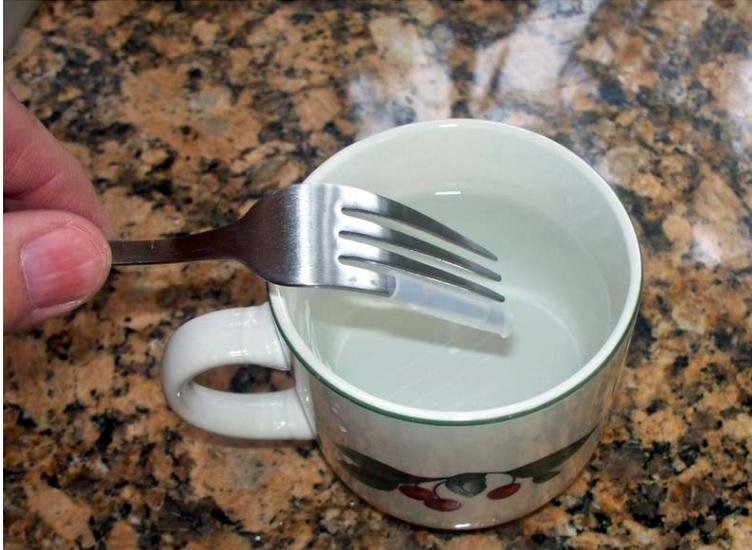
*Heat the coupling in boiling water to make it more pliable*
