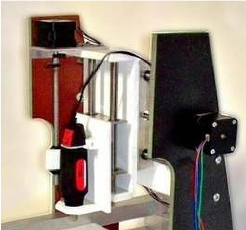
The Z axis/carriage is perhaps the most complex part of the DIY Desktop CNC Machine. Care must be taken to ensure that the Z axis is at exact right angles to the Y axis, and that movement of the Z carriage on the Z axis is smooth.
