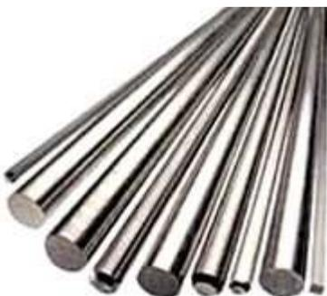
Each axis travels on a pair of  $\frac{3}{8}$ " precision steel rods. It is critical that these rods are smooth and without scratches or nicks as these marks will severely reduce the life of the bearings. Small imperfections may be removed carefully with emery cloth or very fine sandpaper (600 grit or finer). Rods with any blemish that cannot be removed by fine sanding or polishing should be discarded and replaced.
