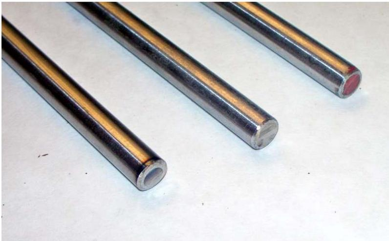
Using a metal file or grinding wheel, chamfer the ends of each cut rod to remove any burrs and to bevel off the shoulder of the cut. This will make it easier to locate each rod in its hole/pocket/grommet without causing damage as the rod is inserted.
