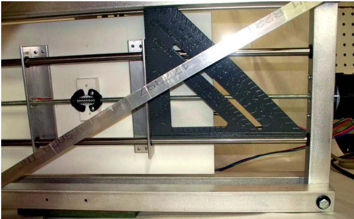
*Use a machinist's or carpenter's square to ensure squareness between the rods and bearing support sub-frames*
