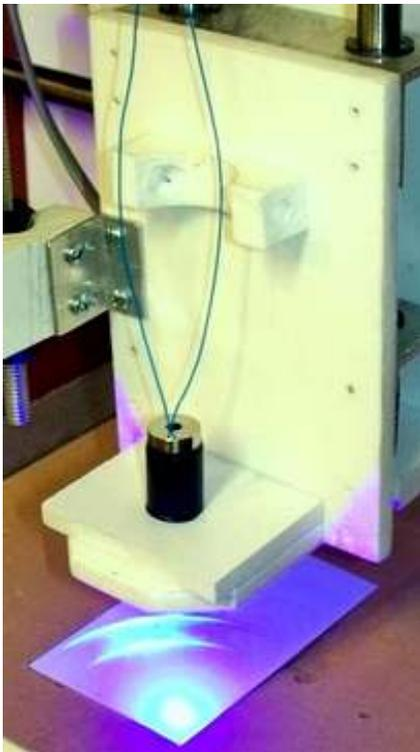
The size and shape of the front (lowest) mount should be made to provide a tight and firm fit. Once cinched down in the upper cradle, the spindle should feel solidly fixed in position without any play or movement between the spindle and the Z carriage.
