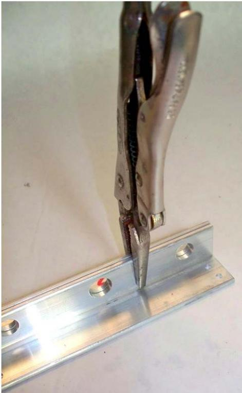
bearing frames to length in pairs. Clamp each pair back to back, as shown in the illustration, ensuring that the pieces are perfectly aligned. Drill the 7/16" holes for the bearings and to clear the threaded rod as shown in the drawings. Mark each pair to keep them together and not mixed up with the other bearing sub frames.
